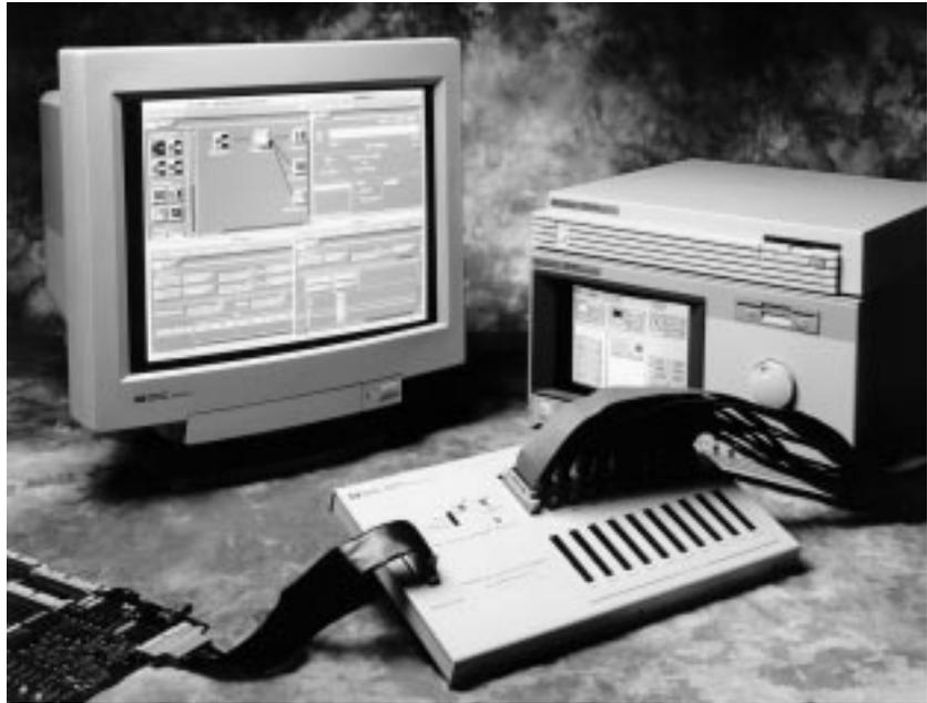
The HP 16500C (right) is the mainframe for measurement modules, such as the HP 16550-series. The HP 16505A prototype analyzer (atop the HP 16500C) combines a large windowed interface with powerful analysis tools. The HP E2485A (foreground) converts up to five HP 16556D modules for up to 40 Mb/channel memory depth.
