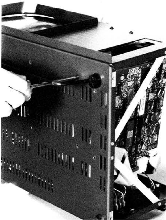
FIG. 4-30 The drives are held in place by additional screws through the chassis.
