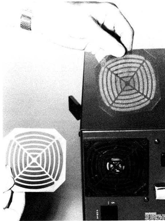
FIG. 7-2 If you are getting some puzzling BIOS errors, check to see if the filter needs cleaning.
