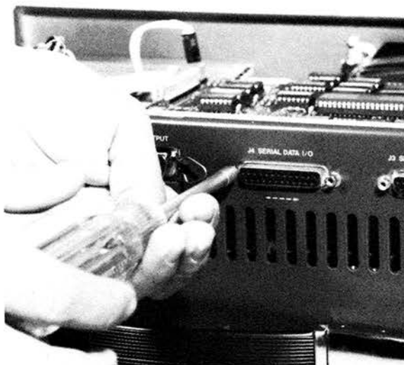
FIG. 5-8 A nut driver is usually needed to remove the screws that hold the ports of the main board.
