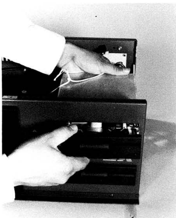
FIG. 8-5 Remove the drive carefully. Some drives have components sticking up that can be damaged.
