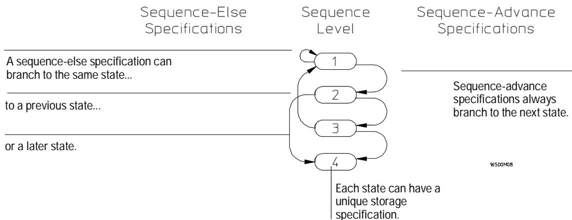
**State Analyzer Sequencer with Four States**
