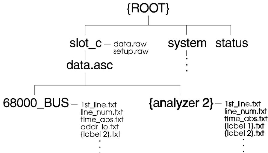
After setting up a measurement and acquiring data, you want to analyze the data for label addr\_lo on your PC. To copy the ASCII data to your local computer, enter the following command at the DOS prompt:
