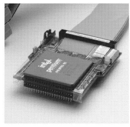
HP microprocessor adapters are compact in design. This Pentium® adapter provides over 160 signal connections to the logic analyzer.
