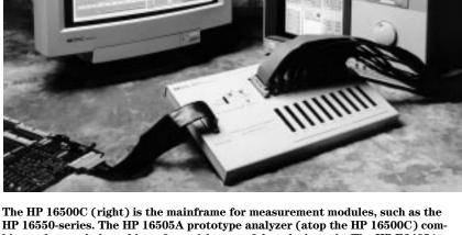
The HP 16500C (right) is the mainframe for measurement modules, such as the HP 16550-series. The HP 16505A prototype analyzer (atop the HP 16500C) combines a large windowed interface with powerful analysis tools. The HP E2485A (foreground) converts up to five HP 16556D modules for up to 40 Mb/channel memory depth.
